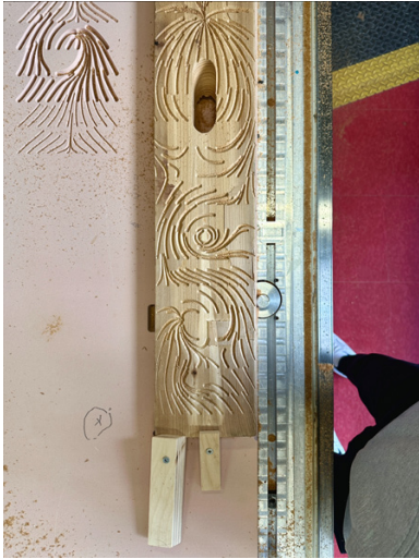
Fig. 5.6.7. CNC milled paddle on machine bed
